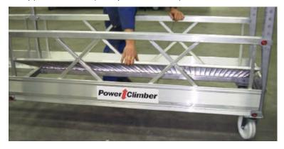
Check that all 4 retaining springs are in place.
