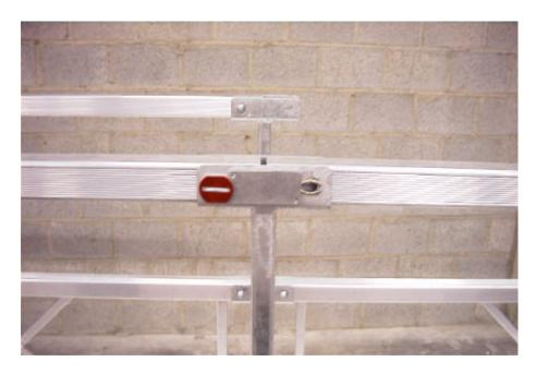
**Remarks:** 1. The guardrail has to be mounted if platform is used.
